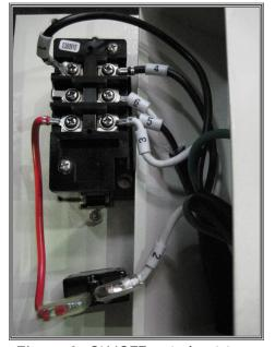
Figure 9. ON/OFF switch wiring.
